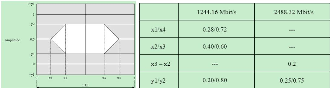
Note 7: Measured with a PRBS 2<sup>23</sup>-1 test pattern @1.244Gbps, BER 1X10<sup>-10</sup>.
